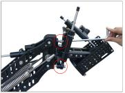
Attach Vibration Isolator with Isolator Section. Insert the bolts from both side of the Isolator Plate then tighten all the Allen bolts with the help of Allen key.
